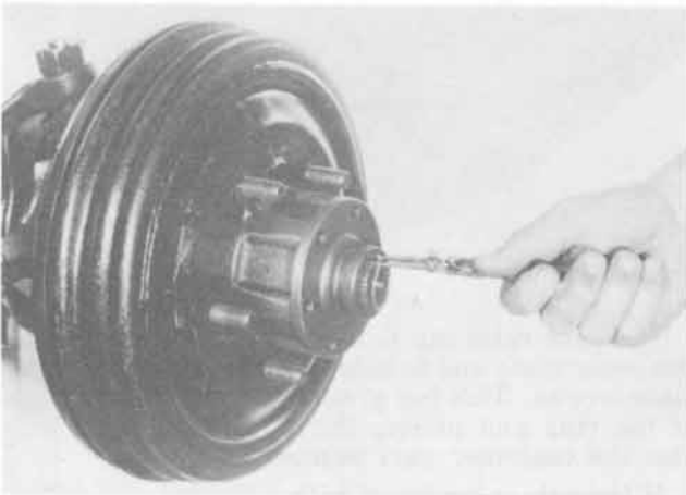
Figure 7 Remove snap ring and drive flange screws.
